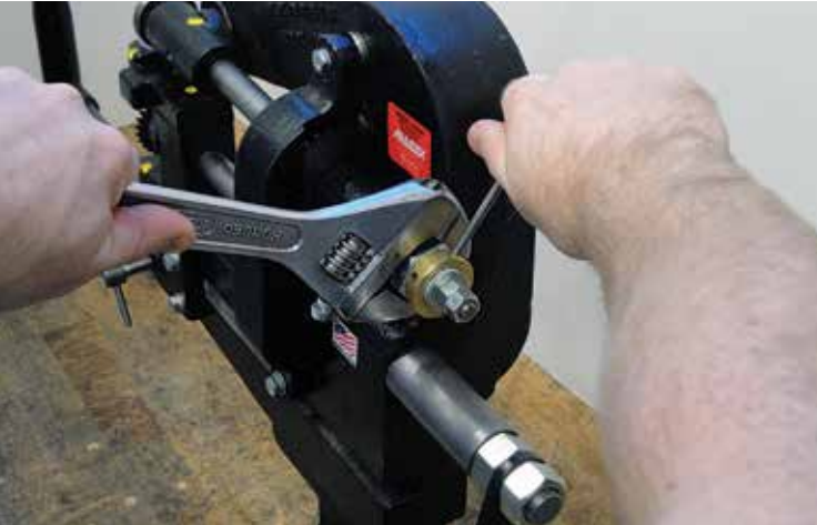
(Figure 14) The correct clearance adjustment for the cutter is achieved by placing a piece of 0.003" shim stock between the top cutting disc and the bottom cutter and adjusting until there is slight resistance on the shim stock.
