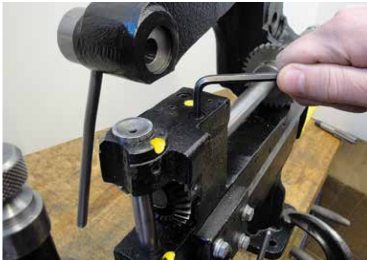
(Figure 10E) Remove bottom cutter support bearing by removing two socket head cap screws holding the bottom cutter support bearing in place. There are two locating pins which align the bottom cutter support bearing to the frame assembly. The pins do not need to be removed, but you may need a non-marking hammer to help ease the bottom cutter support bearing from the frame assembly as the pins fit tightly.
