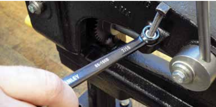
(Figure 15) The depth of cut is adjusted by screwing the depth adjustment screw (I) in, or out, until 1/32" depth of cut is achieved. Lock adjustment screw in place with locking nut using 7/16" wrench.
