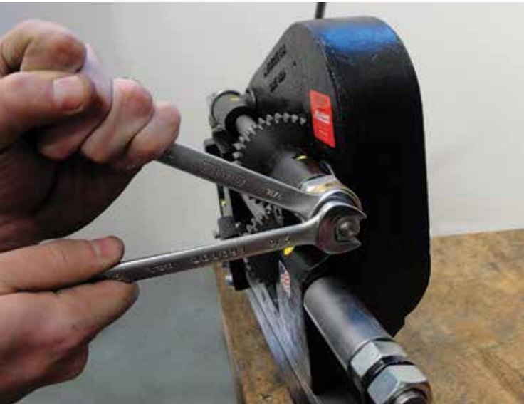
(Figure 13) Remove top shaft assembly end-play by unscrewing the outer hex-nut (F) with 9/16" wrench and adjusting the inner hex-nut (E) in, or out. Once end-play is removed (top shaft assembly will not slide back and forth), lock the inner hex-nut in position. Hold the inner hex-nut with a wrench and tighten the outer hex-nut snug against the inner hex-nut, being careful not to change the position of the inner hex-nut. Double check that end-play has been removed. Crank cutter handle to make sure the top shaft assembly has not been adjusted too tight and that it rotates with just slight resistance.
