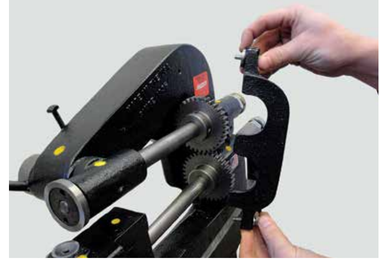
(Figure 10B) Remove gear guard by loosening two hex head cap screws using 7/16" wrench. Pull off gear guard.
