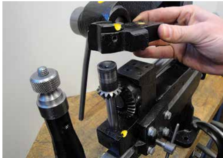
(Figure 10E) Remove bottom cutter support bearing by removing two socket head cap screws holding the bottom cutter support bearing in place. There are two locating pins which align the bottom cutter support bearing to the frame assembly. The pins do not need to be removed, but you may need a non-marking hammer to help ease the bottom cutter support bearing from the frame assembly as the pins fit tightly.
