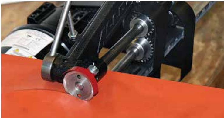
(Figure 7) Hold down momentary switch to engage motor. Simultaneously, with the other hand, maintain a constant downward pressure on the cutting disc lever. As the cutting discs rotate, the gasket material will be drawn towards the cutting discs initiating the cutting process. Continue pressing switch until the entire OD of the gasket material has been cut. Disengage the top cutting disc. Discard unwanted material.
